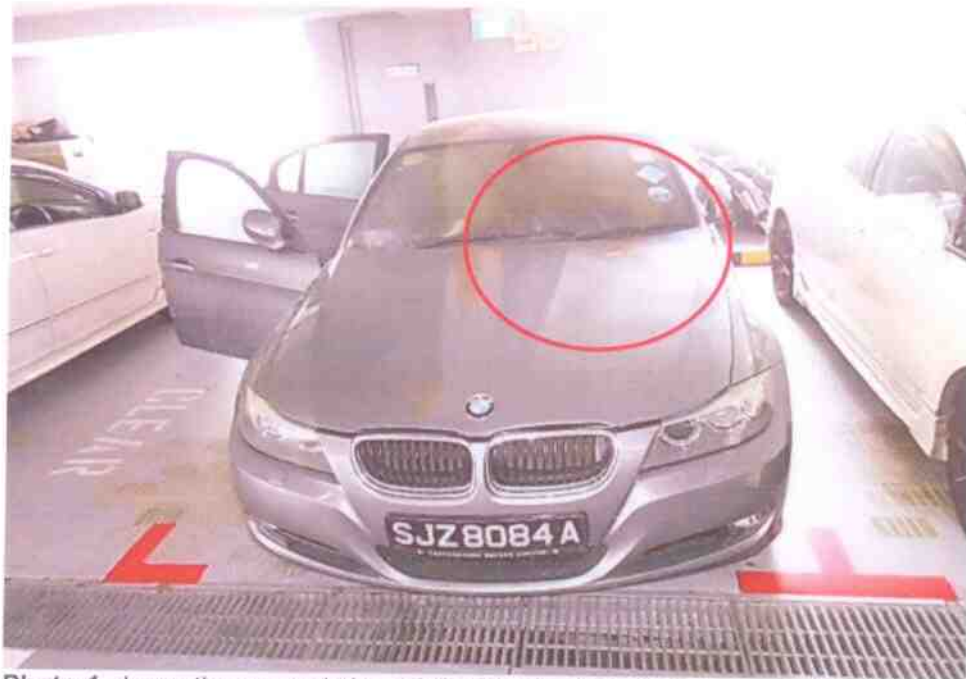
Photo 1 shows the general view of the front portion of the Insured Vehicle at the time of our inspection. The fire damage to the Insured Vehicle was confined to its front bonnet, at the left top area; wiper panel garnish; front windshield; front dashboard and left front door (interior) amongst the body parts that were found to have been affected as a result of the fire.
