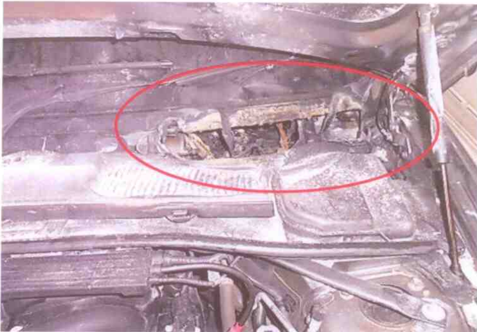
Photo 7 shows a closer view of the wirings around the left rear of the engine compartment, which was in the immediate vicinity where the fire to the Insured Vehicle had likely started.
