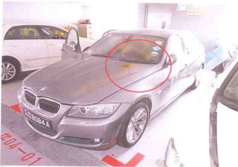
Photo 2 shows the general view of the front left portion of the Insured Vehicle at the time of our inspection. The fire damage to the Insured Vehicle was confined to its front bonnet, at the left top area; wiper panel garnish; front windshield; front dashboard and left front door (interior) amongst the body parts that were found to have been affected as a result of the fire.
