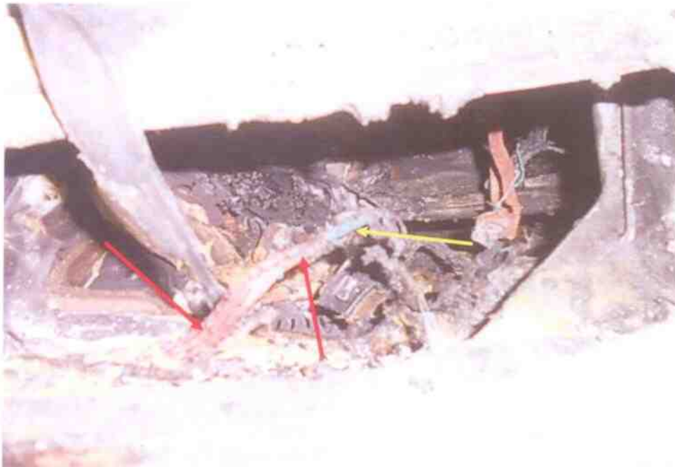
Photo 8 shows a closer view of the wirings (red arrow) which were found to have been burnt internally to its bare copper state, suggesting occurrence of an electrical short circuit. These wirings were observed to be greenish (yellow arrow) believe to be the focal point of the fire ignition.
